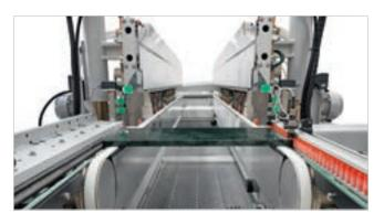
The inlet glass aligning units help the operator to position the glass correctly in the machine, thanks to a proper length of the glass inlet area.
