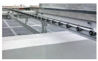
Intermediate bars with automatic positioning function. The positioning of the bar or intermediate bars can be automated; this is recommended when producing small batches.
