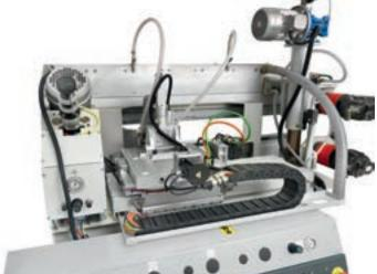
Easy access for the replacement of the grinding wheels, simply by tilting the spindle.
