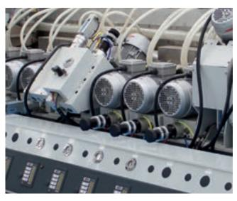
Machine setting times are notably reduced by the proportional valves for automatically managing the pressure on the polishing tools according to the thickness.
